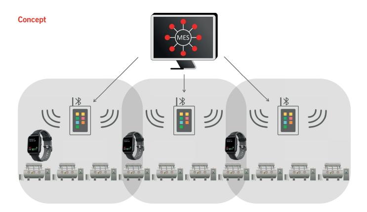
With the Smart Bracelet, operators receive all immediate notifications directly on their wrist even when the operator is not next to the machine. The wristband is connected to the data units which receive operator calls and alarms from SedoMaster. Settings and messages for the Smart Bracelet can be configured and specified for different operators.
